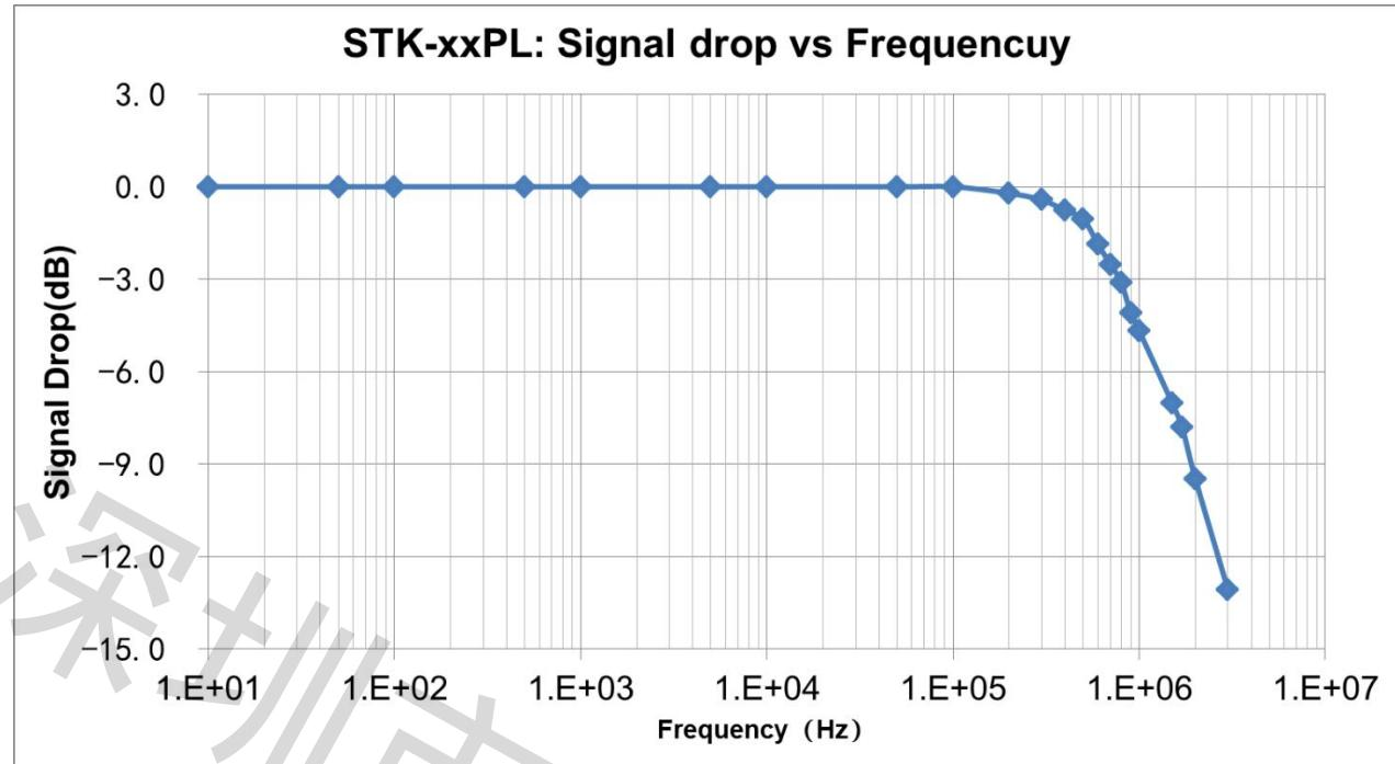
The frequency bandwidth of STK-PL series current sensor. The bandwidth of current sensor is DC ~ 400 kHz (-3dB).
