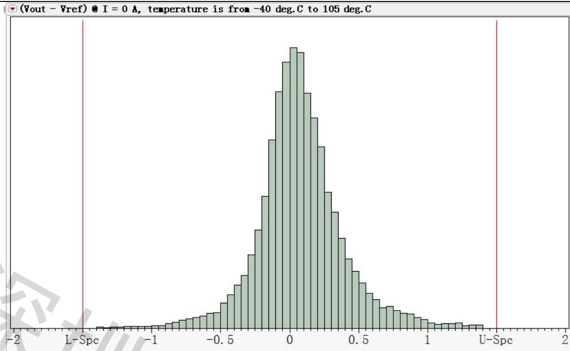
Temperature drift of Voe,  $Voe\_TRange = (Voe @ T_x - Voe @ 25^\circ C) / V_{FS}$ .  $T_x$  represents present temperature,  $V_{FS}$  the rated output voltage.
