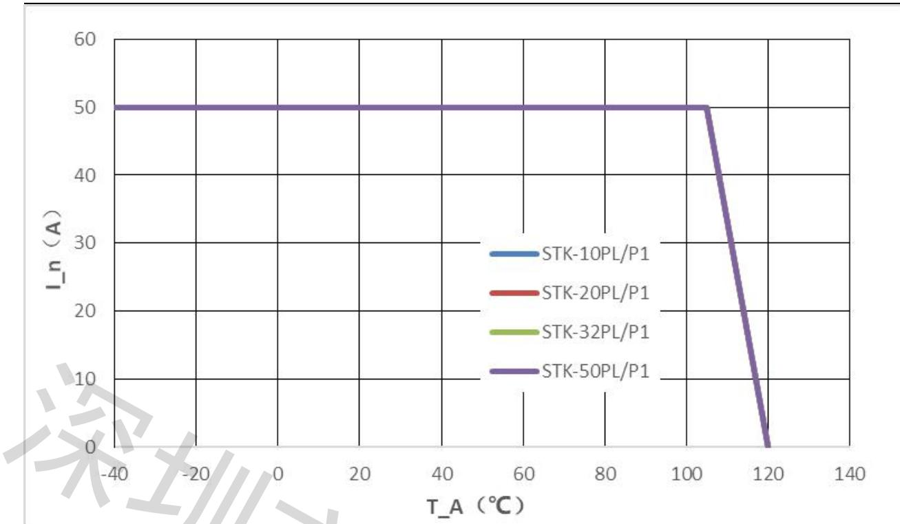
The dependence of maximum continuous current of STK-PL/P1 current on the working temperature
