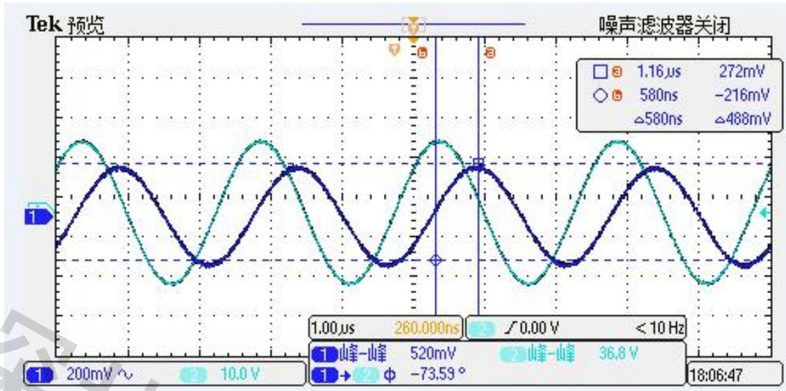
When testing 400kHz sine wave, the typical result of STK-xxPL current sensor's output. The response time from the primary current (light blue) to the secondary output (dark blue) is less than 1  $\mu$ s.
