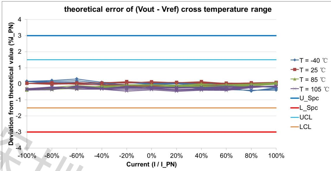
The error of STK-PL current sensor at  $-40^{\circ}\text{C} \sim 105^{\circ}\text{C}$  compared with the standard output at room temperature,  $((V_{out} - V_{ref})_{measure} @ I_n @ T_x - V_{oe} @ T_x - G_{th} * I_n) / V_{FS}$ . Where,  $V_{out}$  represents voltage of  $V_{out}$ ,  $V_{ref}$  the voltage of  $V_{ref}$ ,  $I_n$  the primary current,  $T_x$  the present temperature,  $V_{oe}$  the  $(V_{out} - V_{ref}) @ 0A$ ,  $G_{th}$  the theoretical gain,  $V_{FS}$  the rated output voltage.
